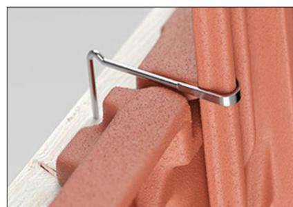
Roof tiles must be clipped and fixed with two screws 4.5 x 45mm with neoprene washers.
